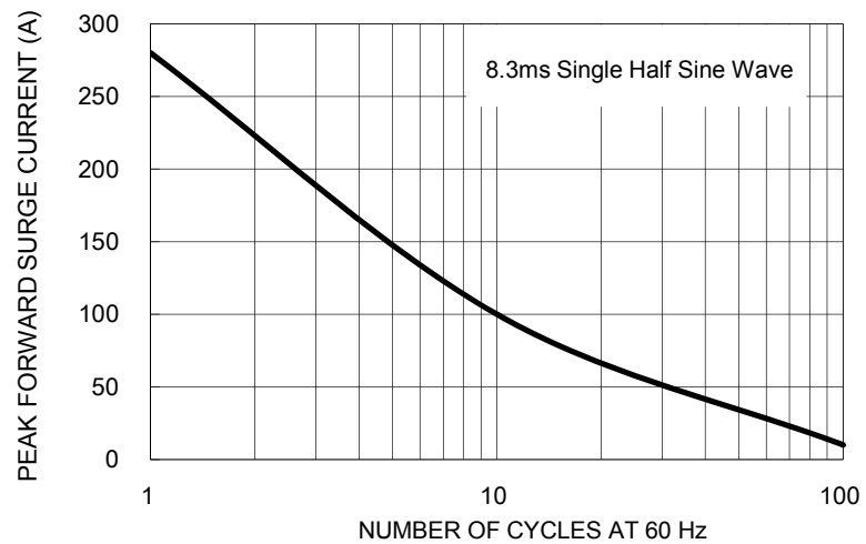
FIG. 5 MAXIMUM NON-REPETITIVE PEAK FORWARD SURGE CURRENT
