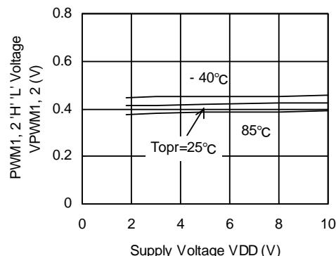
(15) EN1, 2 'H'L' Voltage vs. Supply Voltage
