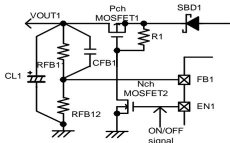
Set R1 so as to prevent leakage current of N-ch MOSFET 2.
