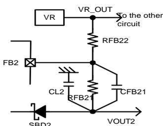
A stable positive voltage produced by a positive voltage regulator or by other means is usable.
