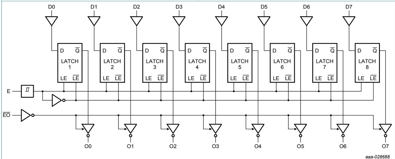
Figure 5. Logic diagram
