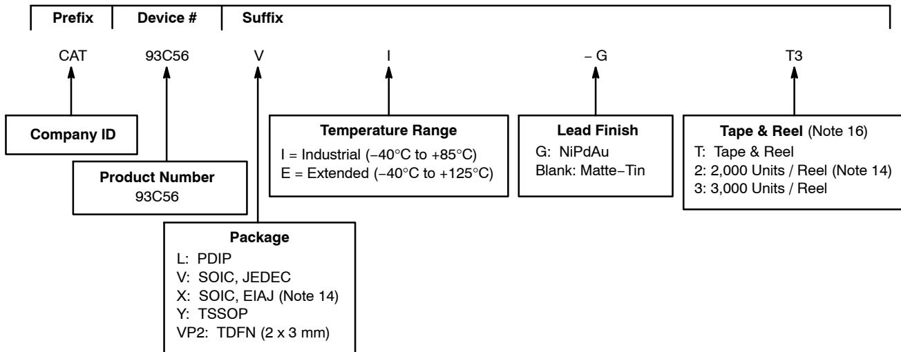
9. The device used in the above example is a CAT93C56VI-GT3 (SOIC, Industrial Temperature, NiPdAu, Tape & Reel).
