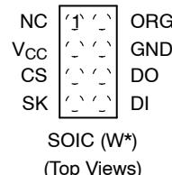
\* TDFN 3x3 mm (ZD4) and SOIC (W) rotated pin-out packages are available for CAT93C57 and CAT93C56, Rev. E only (not recommended for new designs of CAT93C56)
