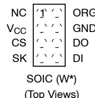
\* TDFN 3x3 mm (ZD4) and SOIC (W) rotated pin-out packages are available for CAT93C57 and CAT93C56, Rev. E only (not recommended for new designs of CAT93C56)
