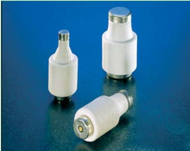
Littelfuse fast acting (gL-gG) fuses are used for the protection of cables against short-circuits. Time-lag (aM) fuses are used for protection of motors. Ratings are available in standard Diazed and compact Neozed styles.
