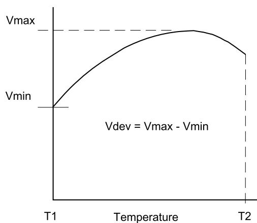
Deviation of reference input voltage,  $V_{dev}$ , is defined as the maximum variation of the reference input voltage over the full temperature range.
