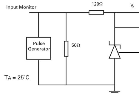
**Test Circuit for Pulse Response**
