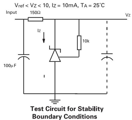
**Test Circuit for Stability Boundary Conditions**
