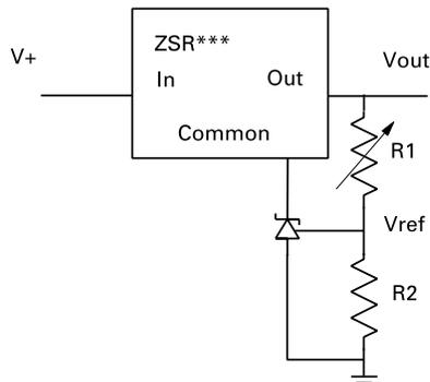
$$V_{out\_MIN} = V_{ref} + V_{reg}$$
