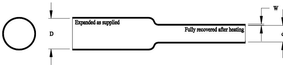
This specification covers the requirements for one type of single wall, electrical insulating, extruded tubing whose diameter will reduce to a predetermined size upon application of heat in excess of 121° C (250° F).
