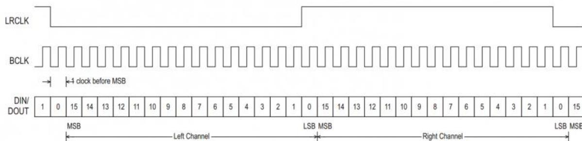
Figure 1. Example I<sup>2</sup>S timing diagram.
