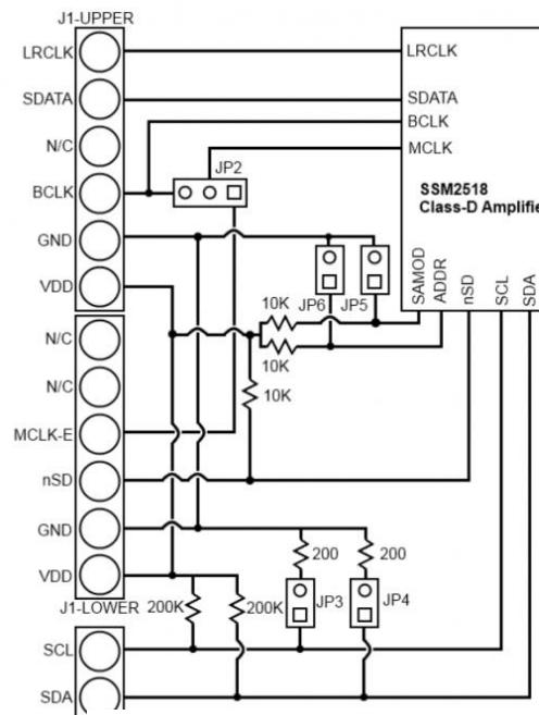
Figure 2. PmodAMP3 block diagram.
