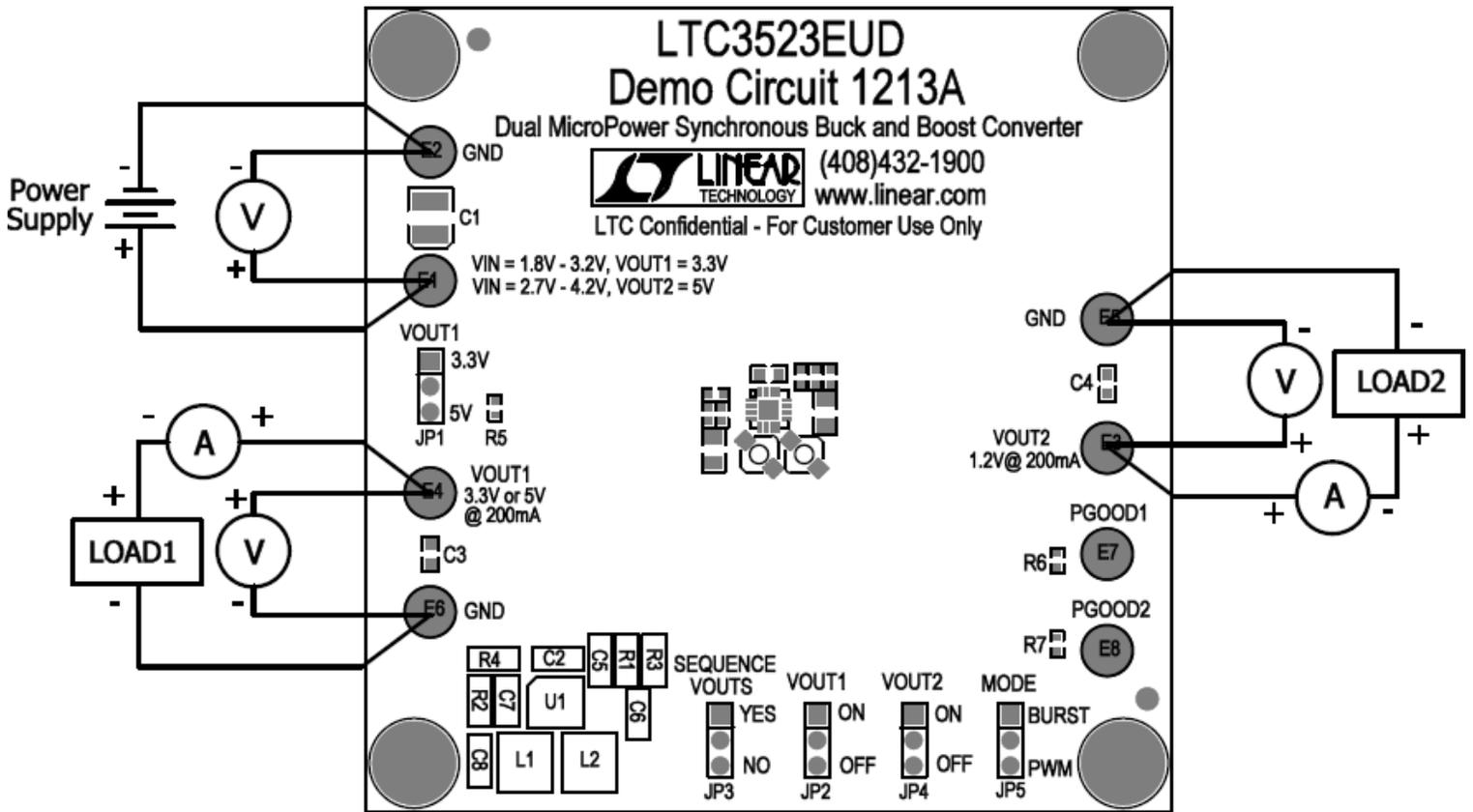
Figure 1. Proper Measurement Equipment Setup
