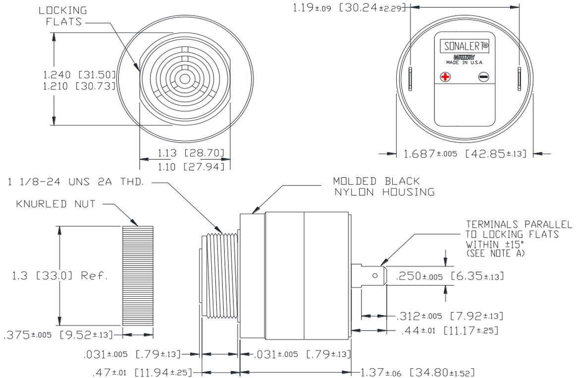
MOUNTING: REMOVE BLACK PLASTIC NUT AND INSERT THREADED FRONT THROUGH 1.25" HOLE PUNCHED IN PANEL, IF ORIENTATION IS NEEDED, NOTE LOCKING FLATS ON DRAWING. SCREW NUT BACK ON. DO NOT OVERTIGHTEN.
