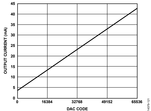
Figure 190. Gain Curve for ANA_FULL_SCALE_CURRENT[9:0] = 1023, DAC Offset = 3.8 mA
