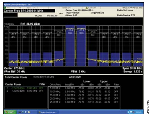
Figure 27. Two-Carrier W-CDMA at 875 MHz
