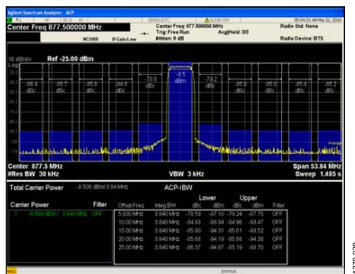
Figure 84. Single-Carrier W-CDMA at 877.5 MHz
