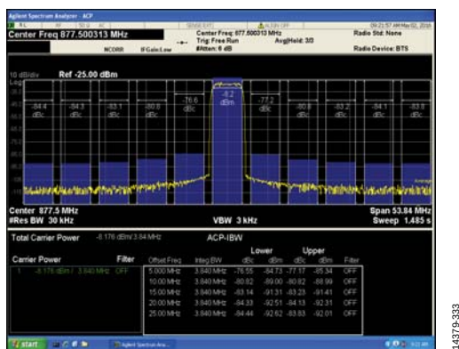
Figure 25. Single-Carrier W-CDMA at 877.5 MHz
