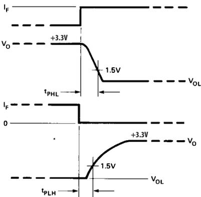
Figure 9 Test Circuit for Transient Immunity and Typical Waveforms
