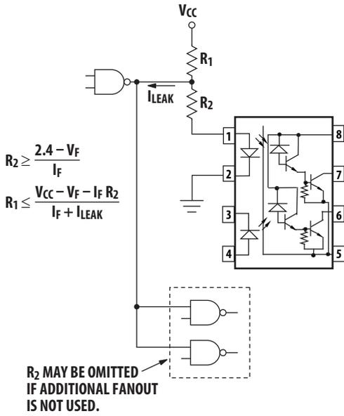
**Figure 11 Operating Circuit for Burn-In and Steady State Life Tests**
