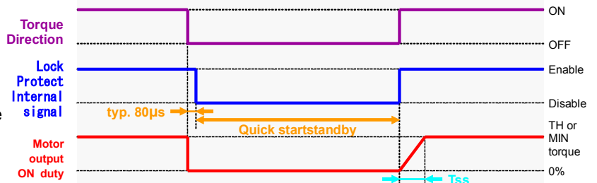
Fig.38 Torque direction and quick start timing chart
