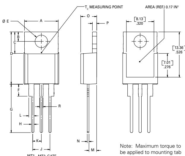
Note: Maximum torque to be applied to mounting tab is 8 in-lbs. (0.904 Nm).
