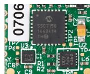
The MM7150 motion module consists of three chips: Bosch BMC150 accelerometer, Bosch BMG160 Gyroscope, and Microchip's SSC7150 motion coprocessor.
