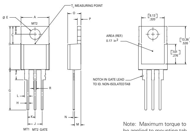
Note: Maximum torque to be applied to mounting tab is 8 in-lbs. (0.904 Nm).
