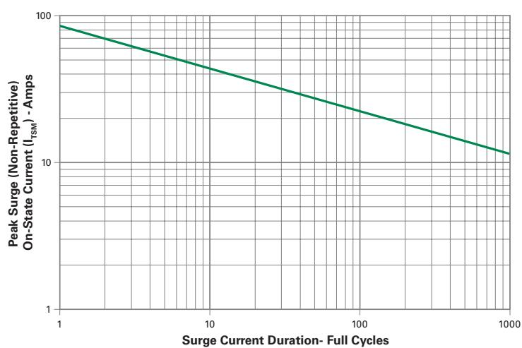
SUPPLY FREQUENCY: 60 Hz Sinusoidal
