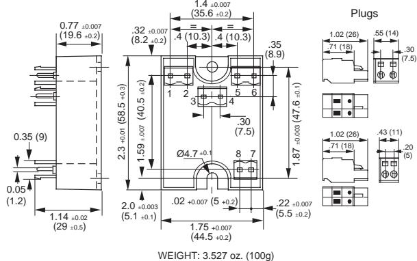
Figure 1 — Series S3P; dimensions in inches (mm)
