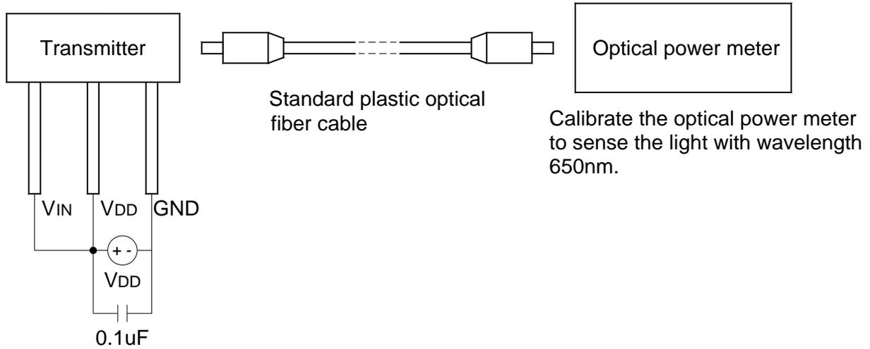
**\*2 Power dissipation measuring method**
