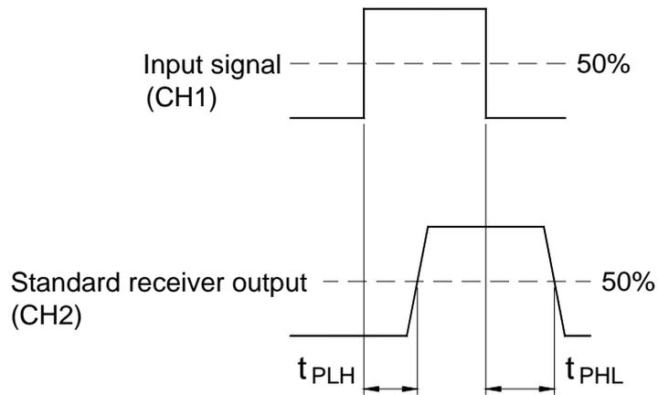
Pulse width distortion  $\Delta tw = t_{PHL} - t_{PLH}$
