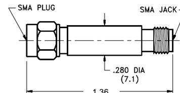
Note: dimensions shown above are for the Male/Female version. The length for the Female/Female version is 1.33 and for the Male/Male version is 1.39.
