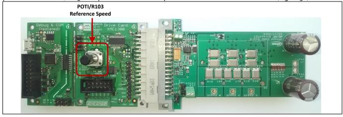
Figure 30 Location of the speed reference control potentiometer POTI/R103
