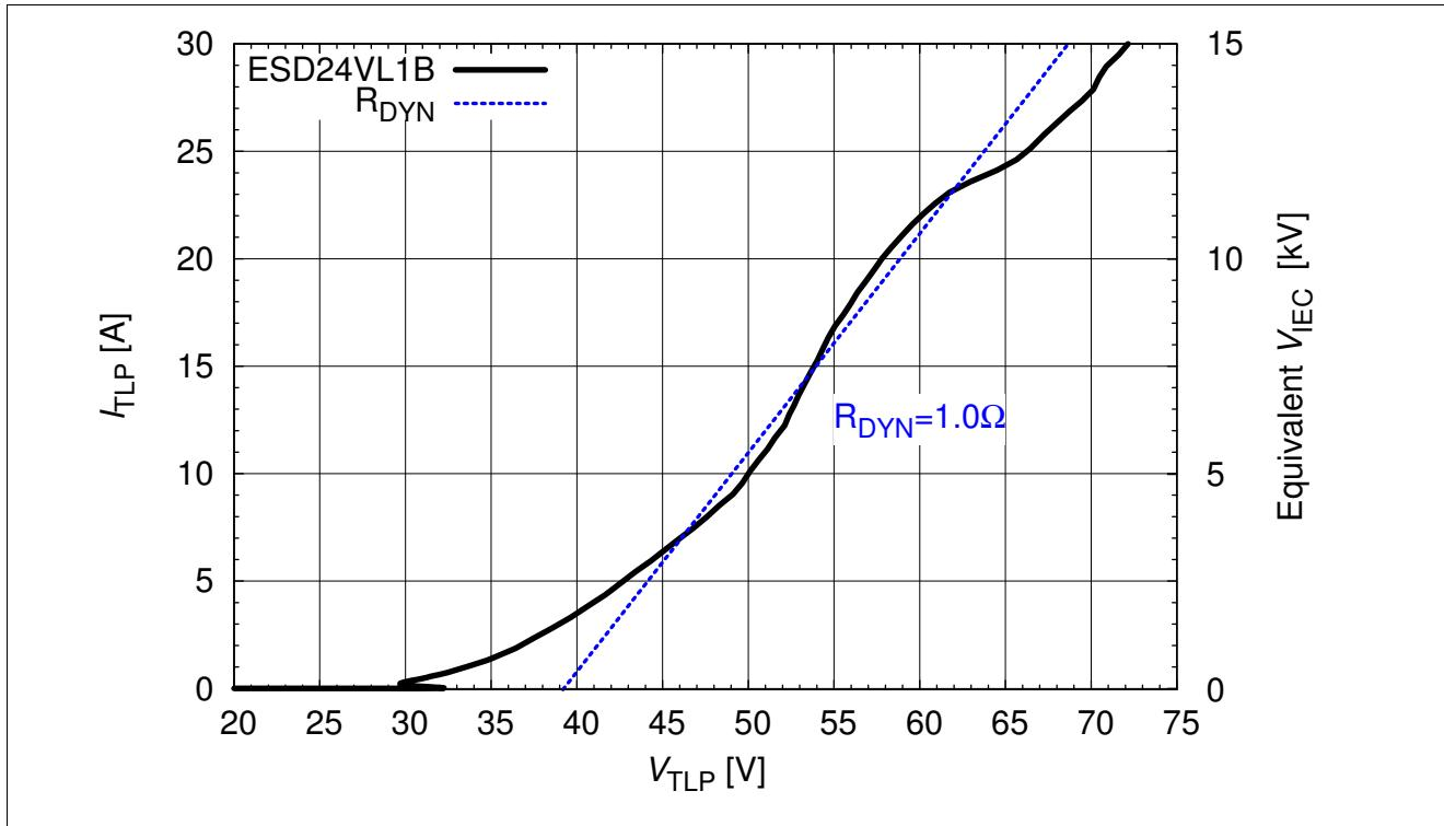
Figure 3-4 Clamping voltage (TLP):  $I_{TLP} = f(V_{TLP})$  [1]
