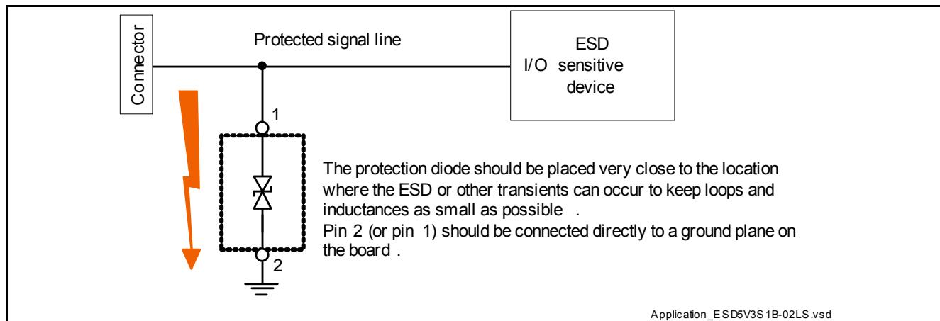
Figure 4-1 Single line, bi-directional ESD / Transient protection
