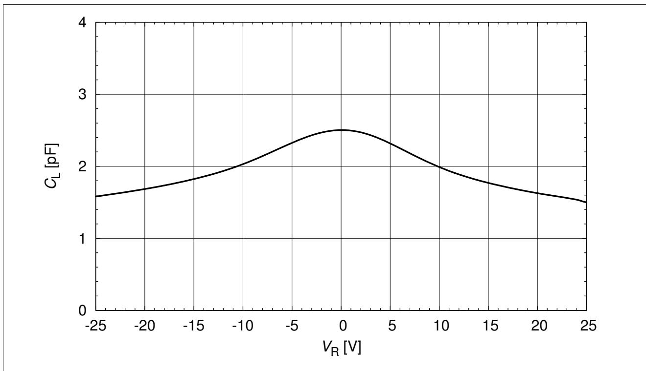
Figure 3-3 Line capacitance:  $C_L = f(V_R), f = 1\text{MHz}$
