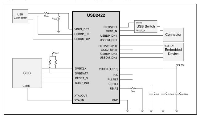
FIGURE 2-6: EXAMPLE APPLICATION - NON-SOC BASED DESIGN
