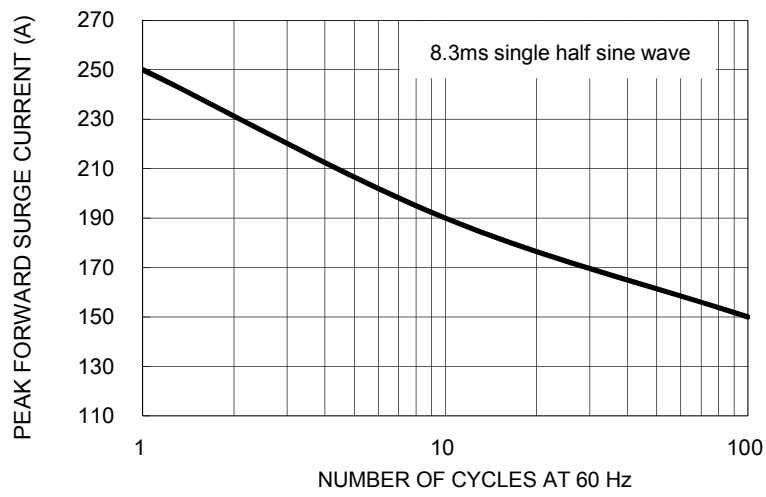
FIG. 7 MAXIMUM NON-REPETITIVE PEAK FORWARD SURGE CURRENT
