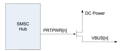
Figure 8.1 Battery Charging External Power Supply
