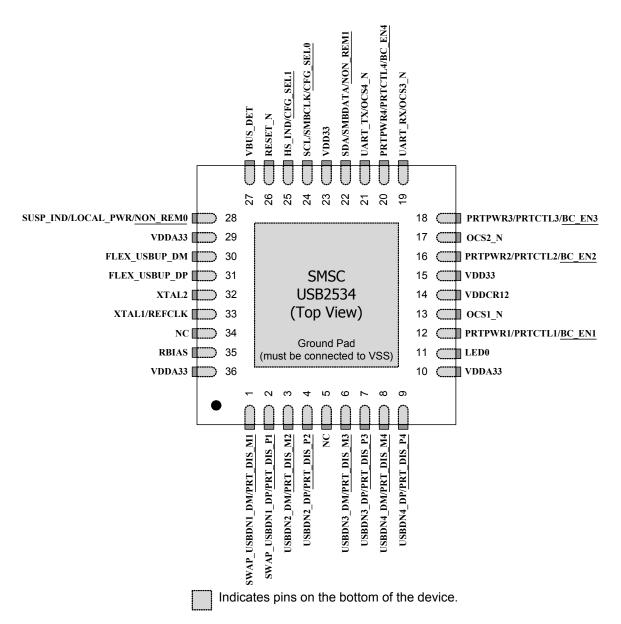
Figure 3.1 36-SQFN Pin Assignments
