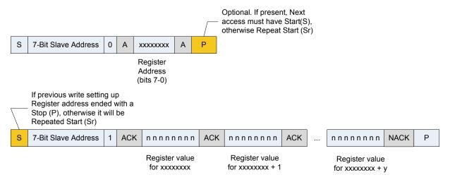
Figure 7.2 I<sup>2</sup>C Sequential Access Read Format
