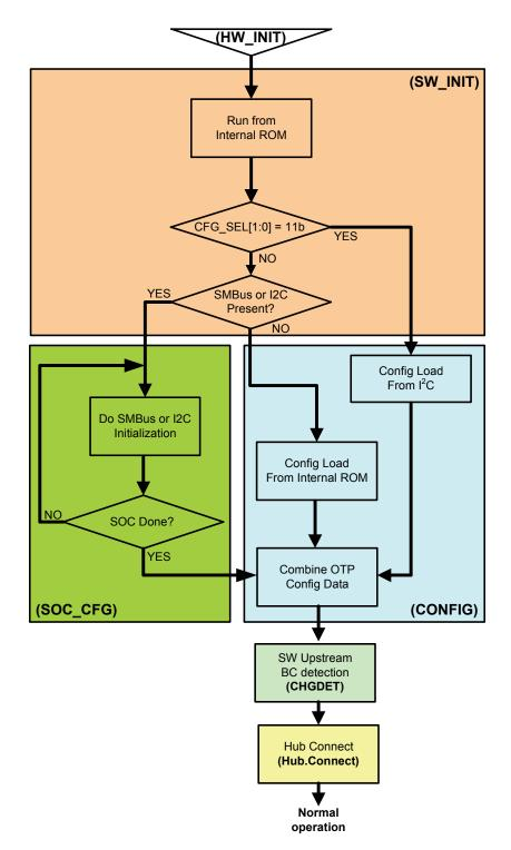
Figure 5.1 Hub Operational Mode Flowchart
