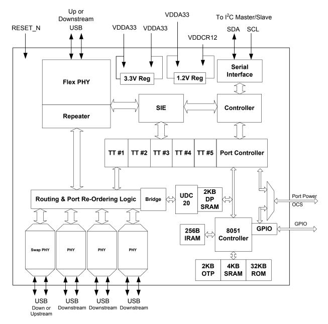
Figure 1.1 System Block Diagram
