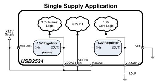
**Figure 4.1 Power Connections**
