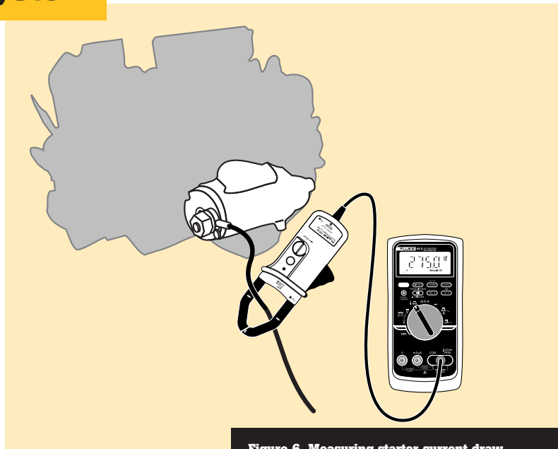
Figure 6. Measuring starter current draw
