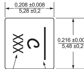
Dash number indicates direction of terminals and start (short) lead. Connect high dv/dt here for lowest EMI.
