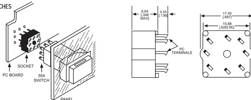
Material: All plastic switch components made from 94V-0 plastic
