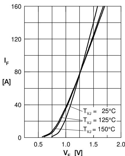
Fig. 1 Forward current versus voltage drop per diode
