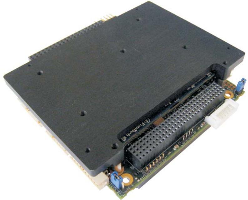
The ISIS XL processor board provides all the benefits of Intel's new Atom LPIA architecture in a PC/104+ form factor; comprising of a processor module and carrier board.
