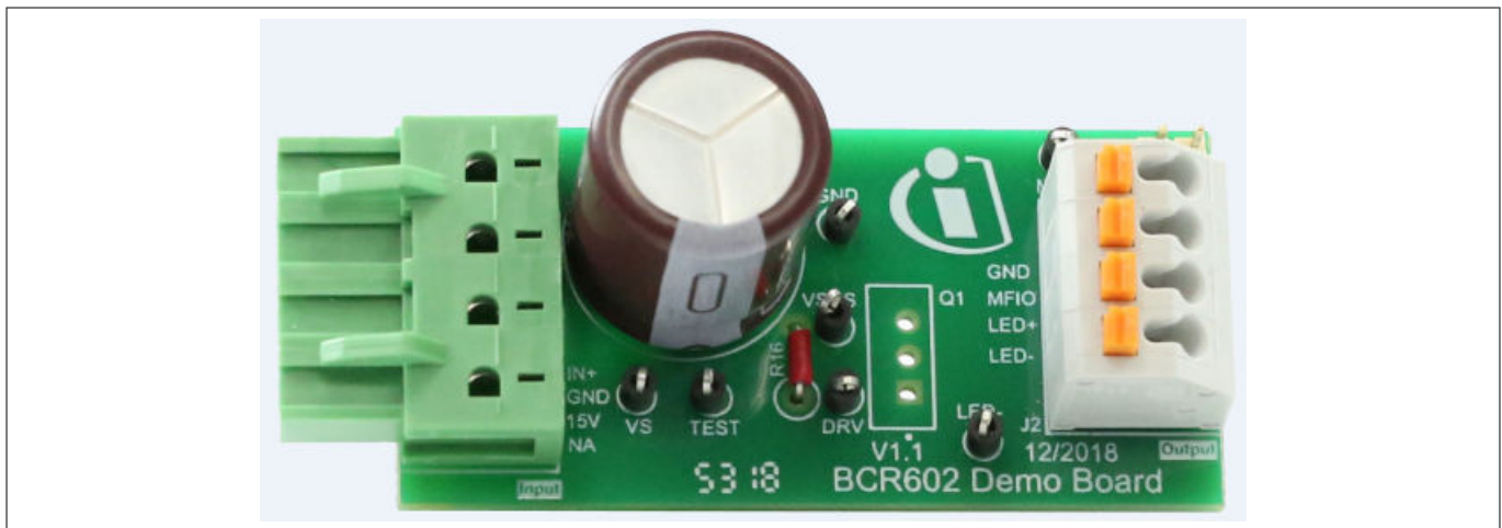
Figure 2 Top side of the demonstrator design board (56.00 mm x 27.00 mm)
