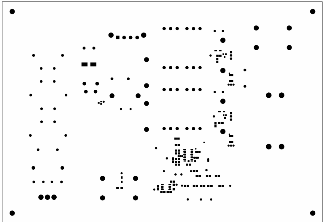
Figure 9. Top Solder Mask
