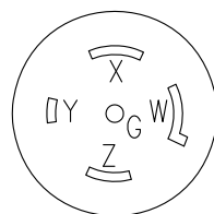
DETAIL B (NEMA L21-20P PLUG-ENLARGED)
