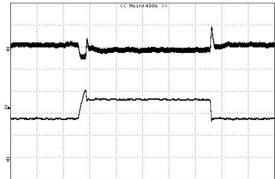
Figure 9: Output voltage response to step-change in load current (75%-50%-75% of I_o , max; di/dt = 1.0A/\mu s ). Load cap: 470uF POS capacitor and 1 \mu F ceramic capacitor. Top Trace: V_{out} (100mV/div, 200us/div), Bottom Trace: I_{out} (10A/div). Scope measurement should be made using a BNC cable (length shorter than 20 inches). Position the load between 51 mm to 76 mm (2 inches to 3 inches) from the module
