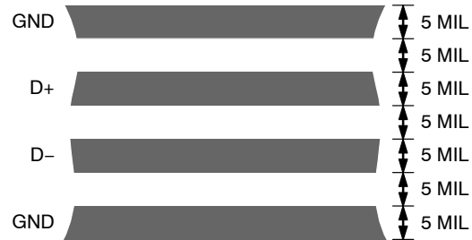
Figure 34. Typical Arrangement of Signal Tracks
