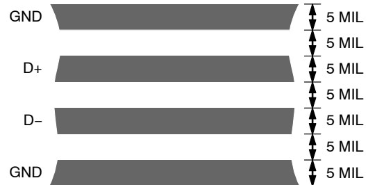
Figure 34. Typical Arrangement of Signal Tracks
