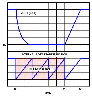
FIGURE 3. OVERCURRENT PROTECTION RESPONSE
