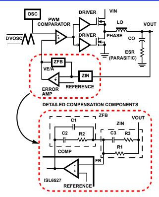
FIGURE 5. VOLTAGE-MODE BUCK CONVERTER COMPENSATION DESIGN
