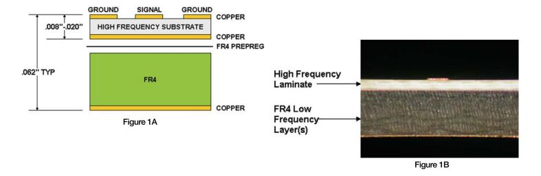
Typical HF/Digital Multilayer Hybrid Construction (GCPW Figure 1A, microstrip Figure 1B)
