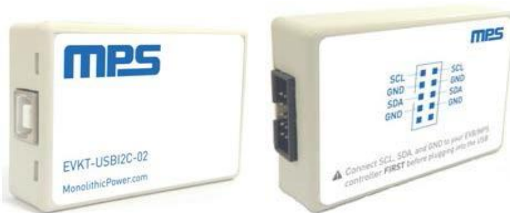
Figure 3: EVKT-USBI2C-02 Communication Interface
