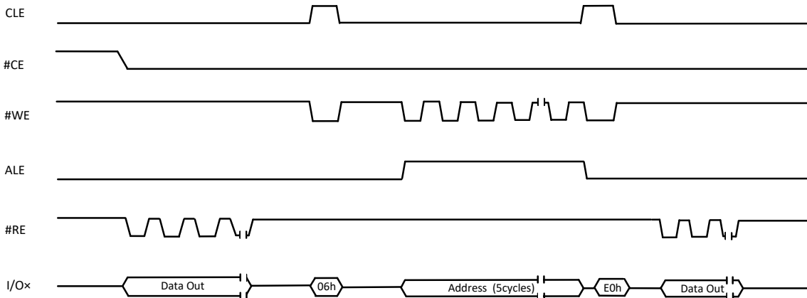
Figure 9-4 Two Plane Random Data Read (06h-E0h) Operation
