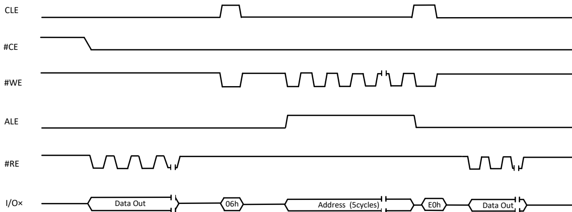
Figure 9-4 Two Plane Random Data Read (06h-E0h) Operation
