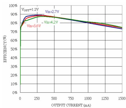
Fig. 7: Efficiency vs Output Current
