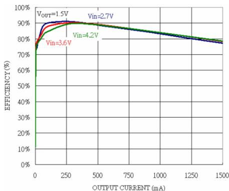
Fig. 6: Efficiency vs Output Current
