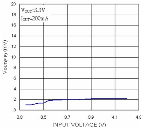
Fig. 24: Output Voltage Ripple in LDO mode
