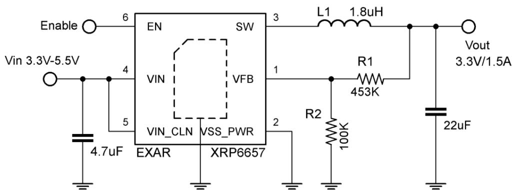
Fig. 1: XRP6657 Application Diagram
