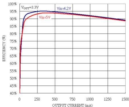
Fig. 4: Efficiency vs Output Current
