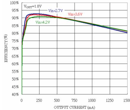
Fig. 5: Efficiency vs Output Current
