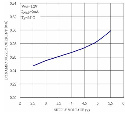
Fig. 15: Dynamic Supply Current vs Supply Voltage
