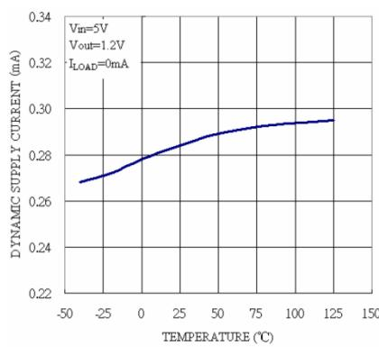
Fig. 14: Dynamic Supply Current vs Temperature
