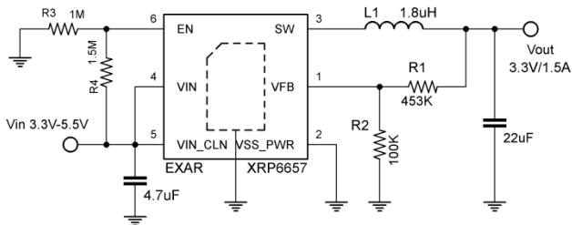
A resistor ratio  $R_3/R_4=1/1.5$  is recommended.
