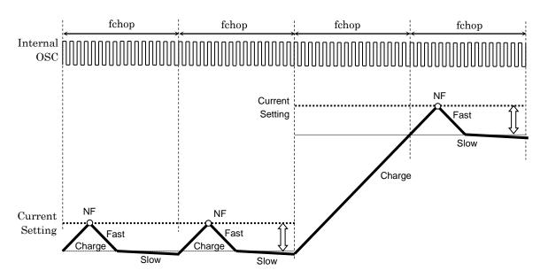
When the Charge period is longer than fchop cycle, the Charge period will be extended until the motor current reaches the NF threshold. Once the current reaches the next current step, then the sequence will go on to decay mode.
