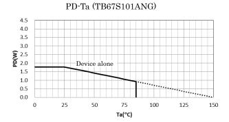
The power dissipation depends on the PCB layout and mounting conditions so please becareful. Also, when the ambient temperature is high, the allowed power disspation will be smaller.
