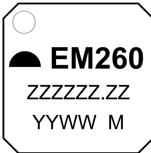
Figure 22. Part marking for EM260
