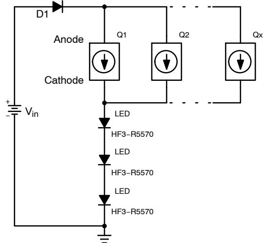
**Figure 8. Typical Application Circuit
