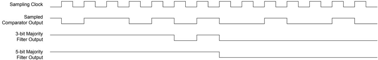
**Figure 36-7. Single-Shot Filtering**
