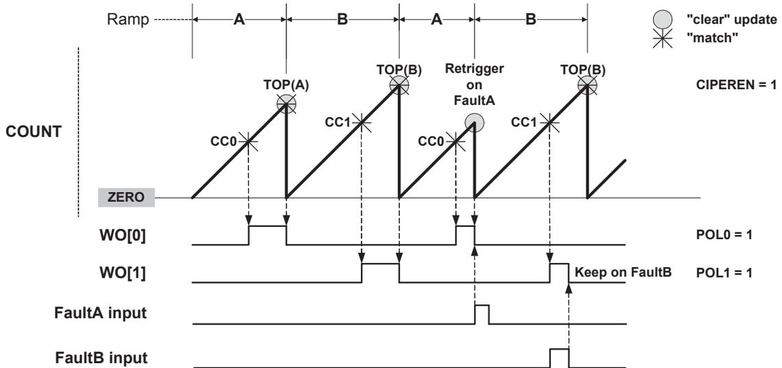
**Alternate RAMP2 (RAMP2A) Operation**
