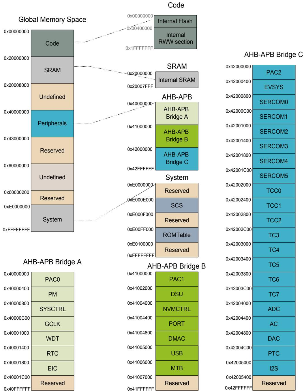
This figure represents the full configuration of the SAM DA1 with maximum flash and SRAM capabilities and a full set of peripherals.
