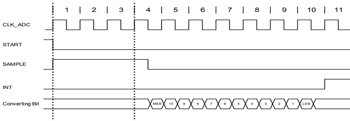
Figure 35-5. ADC Timing for Free Running in Differential Mode without Gain
