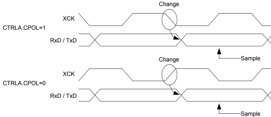
When the clock is provided through XCK (CTRLA.MODE=0x0), the shift registers operate directly on the XCK clock. This means that XCK is not synchronized with the system clock and, therefore, can operate at frequencies up to the system frequency.
