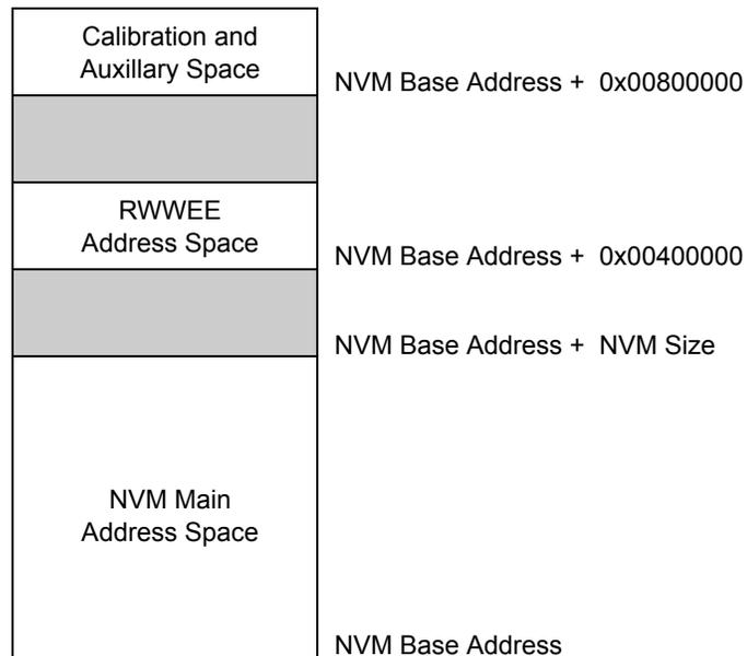
The lower rows in the NVM main address space can be allocated as a boot loader section by using the BOOTPROT fuses, and the upper rows can be allocated to EEPROM, as shown in the figure below.
