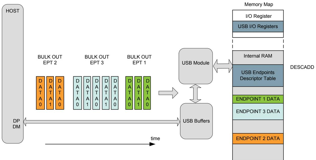
When an OUT token is detected, and the device address of the token packet does not match DADD.DADD, the packet is discarded and the USB module returns to idle and waits for the next token packet.
