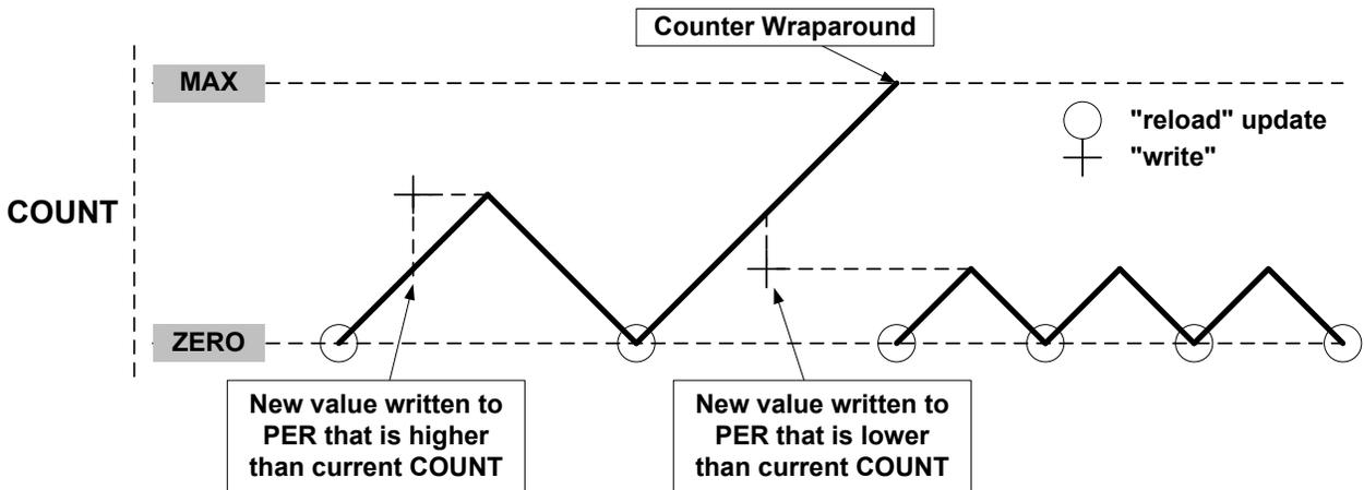
When double buffering is used, the buffer can be written at any time and the counter will still maintain correct operation. The period register is always updated on the update condition, as shown in [Figure 33-13](#). This prevents wraparound and the generation of odd waveforms.
