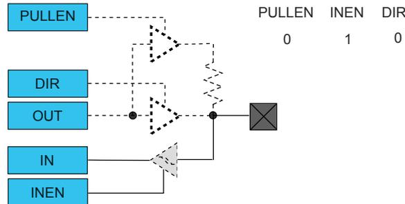
Figure 25-5. I/O Configuration - Input with Pull
