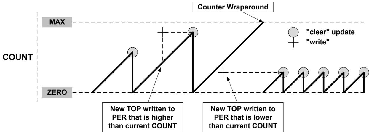
Figure 32-8. Changing the Top Value with Down-Counting Operation
