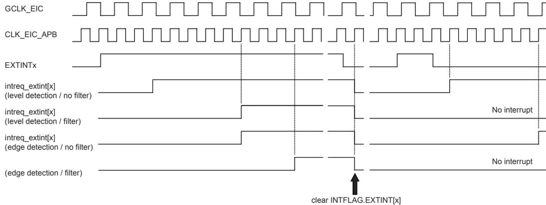
The detection delay depends on the detection mode.
