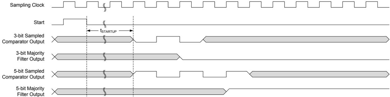
During sleep modes, filtering is supported only for single-shot measurements. Filtering must be disabled if continuous measurements will be done during sleep modes, or the resulting interrupt/event may be generated incorrectly.
