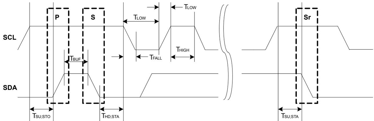
The following parameters are timed using the SCL low time period  $T_{LOW}$ . This comes from the Master Baud Rate Low bit group in the Baud Rate register (BAUD.BAUDLOW). When BAUD.BAUDLOW=0, or the Master Baud Rate bit group in the Baud Rate register (BAUD.BAUD) determines it.
