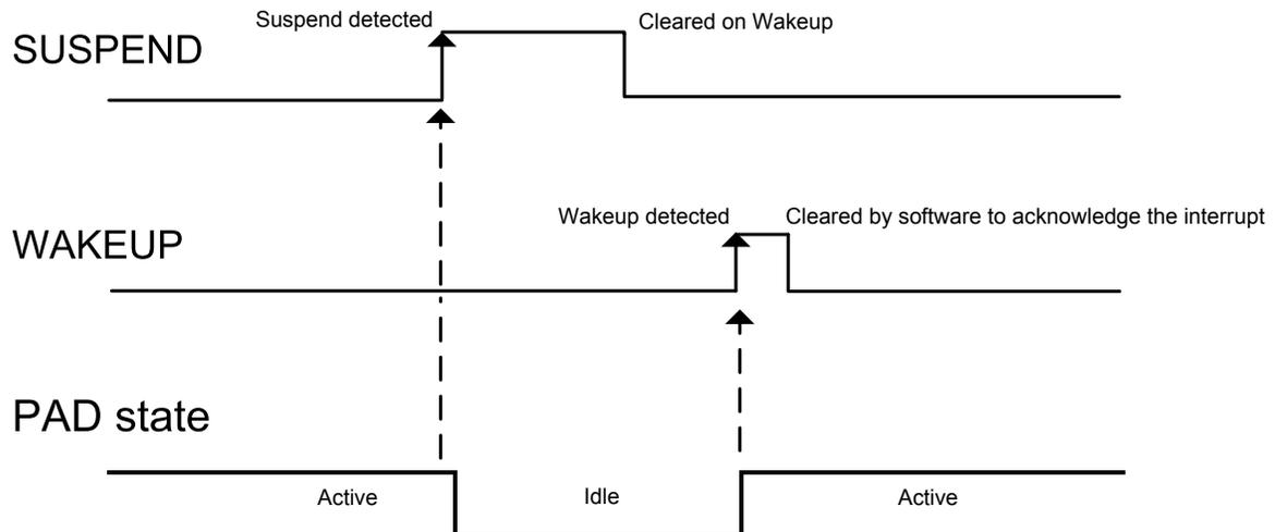
The Suspend Interrupt bit in the Device Interrupt Flag register (INTFLAG.SUSPEND) is set when a USB Suspend state has been detected on the USB bus. The USB pad is then automatically put in the Idle state. The detection of a non-idle state sets the Wake Up Interrupt bit in INTFLAG (INTFLAG.WAKEUP) and wakes the USB pad.
