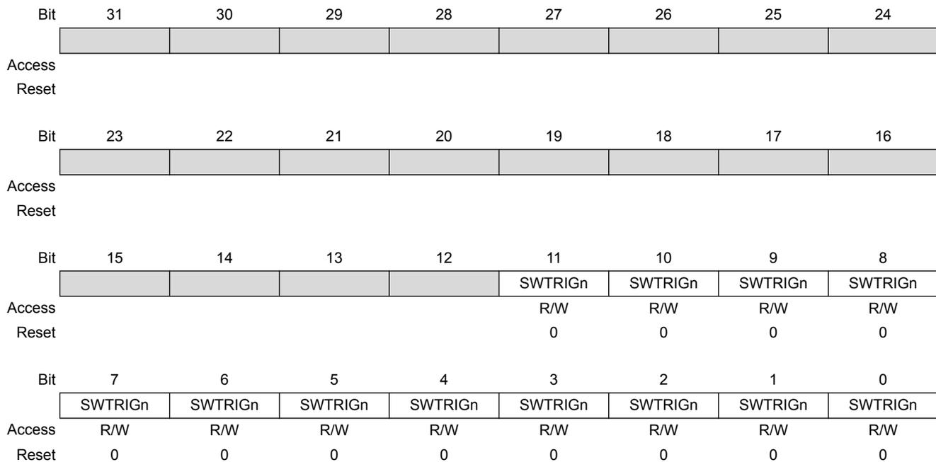
**Bits 11:0 – SWTRIGn: Channel n Software Trigger [n = 11..0]**
