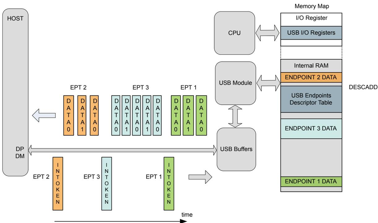
When an IN token is detected, and if the device address of the token packet does not match DADD.DADD, the packet is discarded and the USB module returns to idle and waits for the next token packet.
