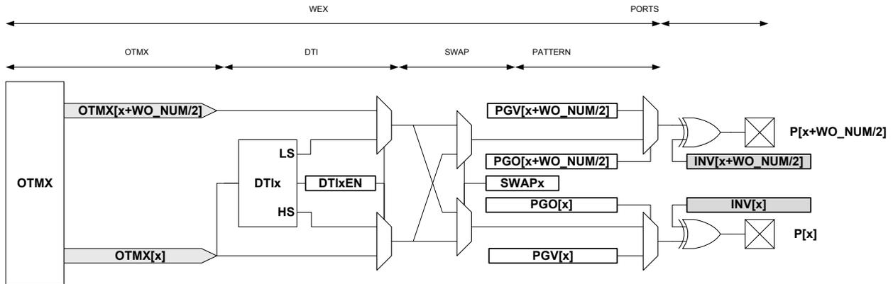
The output matrix (OTMX) unit distributes compare channels, according to the selectable configurations in Table 33-4.
