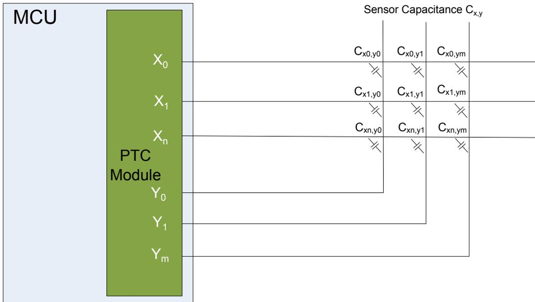
**38.5.1.2 Self-Capacitance Sensor Arrangement**
