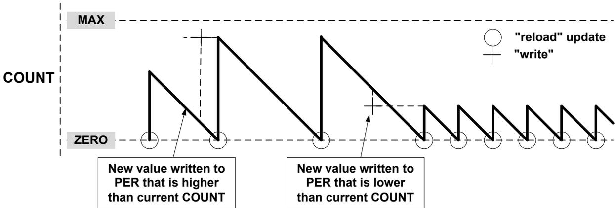
A counter wraparound can occur in any operation mode when up-counting without buffering, see [Figure 33-10](#). COUNT and TOP are continuously compared, so when a new value that is lower than the current COUNT is written to TOP, COUNT will wrap before a compare match.
