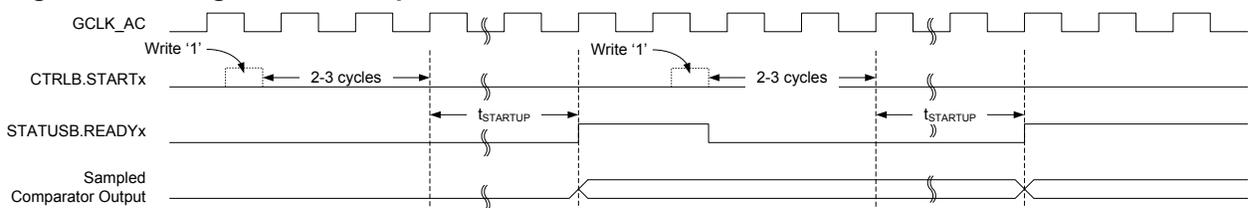
For low-power operation, event-triggered measurements can be performed during sleep modes. When the event occurs, the Power Manager will start CLK\_AC\_DIG. The comparator is enabled, and after the startup time has passed, a comparison is done and appropriate peripheral events and interrupts are also
