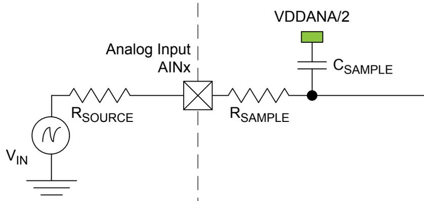
To achieve n bits of accuracy, the  $C_{\text{SAMPLE}}$  capacitor must be charged at least to a voltage of
