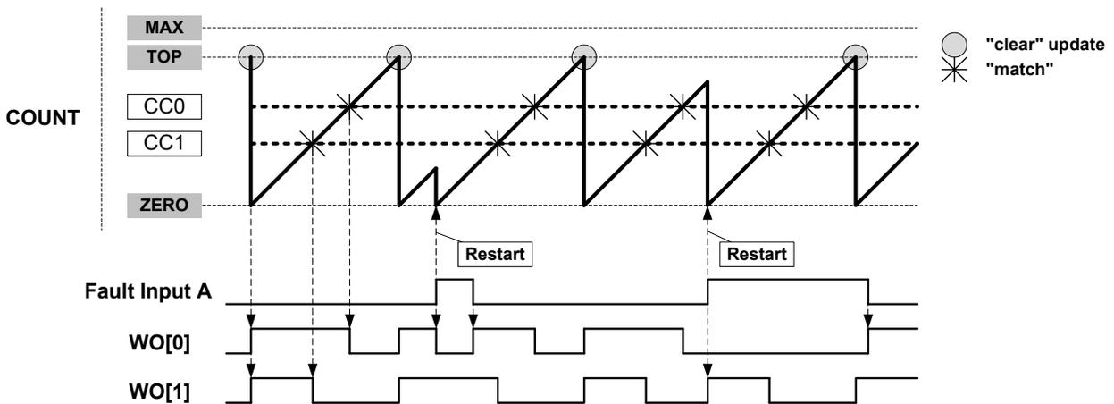
Figure 33-25. Waveform Generation in RAMP2 mode with Restart Action
