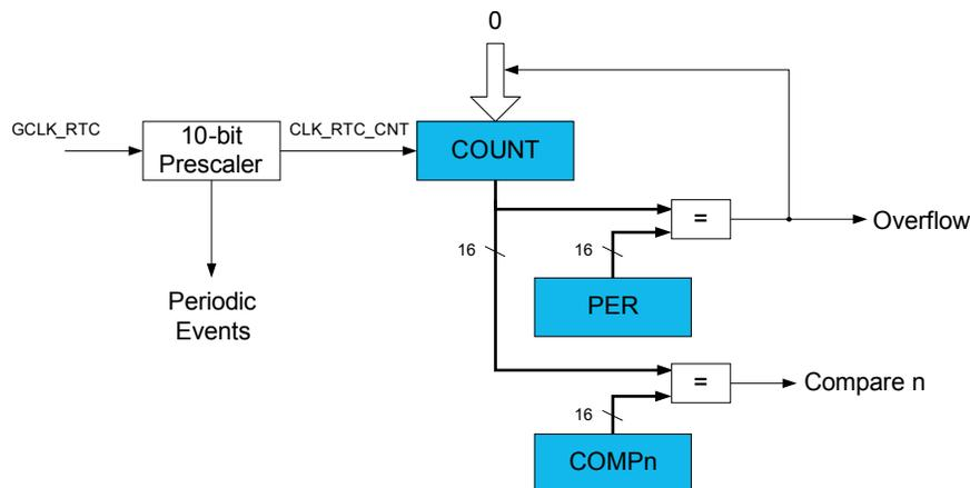
Figure 21-3. RTC Block Diagram (Mode 2 — Clock/Calendar)
