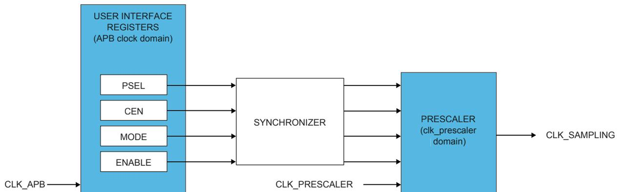
The BOD33 Clock Enable bit (BOD33.CEN) in the BOD33 register and the BOD12 Clock Enable bit (BOD12.CEN) in the BOD12 register should always be disabled before changing the prescaler value. To change the prescaler value for the BOD33 or BOD12 during sampling mode, the following steps need to be taken:
