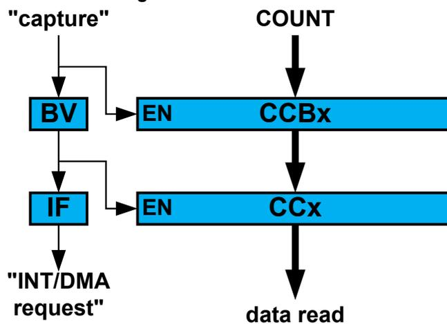
The TCC can detect capture overflow of the input capture channels: When a new capture event is detected while the Capture Buffer Valid flag (STATUS.CCBV) is still set, the new timestamp will not be stored and INTFLAG.ERR will be set.
