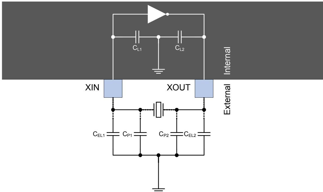
Using this model the total capacitive load for the crystal can be calculated as shown in the equation below:
