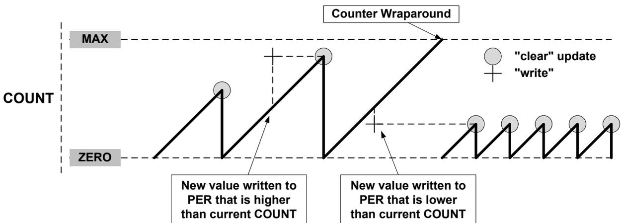
Figure 33-11. Unbuffered Single-Slope Down-Counting Operation
