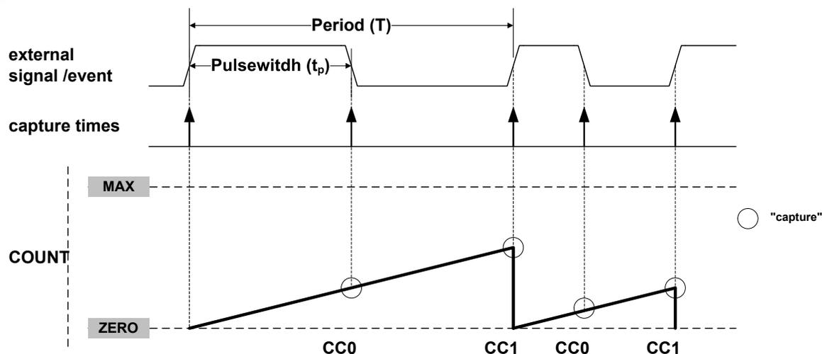
Selecting PWP or PPW in the Timer/Counter Event Input 1 Action bit group in the Event Control register (EVCTRL.EVACT1) enables the TCC to perform one capture action on the rising edge and the other one on the falling edge. When using PPW (period and pulse-width) event action, period  $T$  will be captured into CC0 and the pulse-width  $t_p$  into CC1. The PWP (Pulse-width and Period) event action offers the same functionality, but  $T$  will be captured into CC1 and  $t_p$  into CC0.
