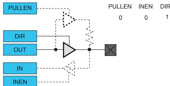
Figure 25-7. I/O Configuration - Totem-Pole Output with Enabled Input
