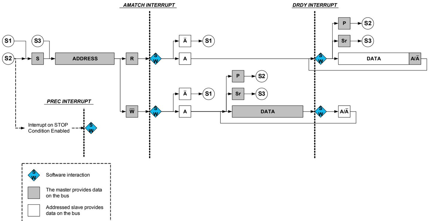
In the second strategy (CTRLA.SCLSM=1), interrupts only occur after the ACK bit is sent as shown in [Slave Behavioral Diagram \(SCLSM=1\)](#). This strategy can be used when it is not necessary to check
