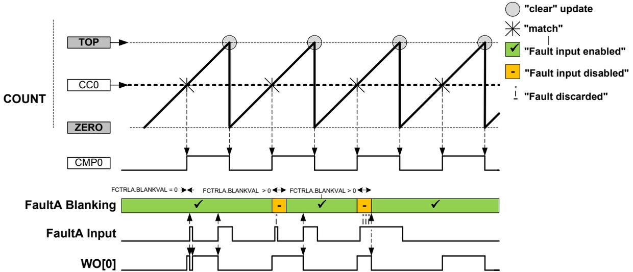
**Fault Qualification** This is enabled by writing a '1' to the Fault n Qualification bit in the Recoverable Fault n Configuration register (FCTRLn.QUAL). When the recoverable fault qualification is enabled (FCTRLn.QUAL=1), the fault input is disabled all the time the corresponding channel output has an inactive level, as shown in the figures below.
