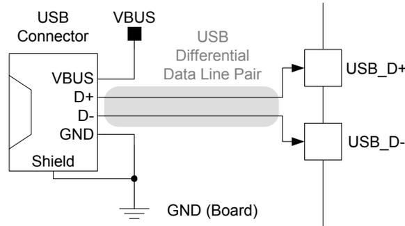
It is recommended to increase ESD protection on the USB D+, D-, and VBUS lines using dedicated transient suppressors. These protections should be located as close as possible to the USB connector to reduce the potential discharge path and reduce discharge propagation within the entire system.
