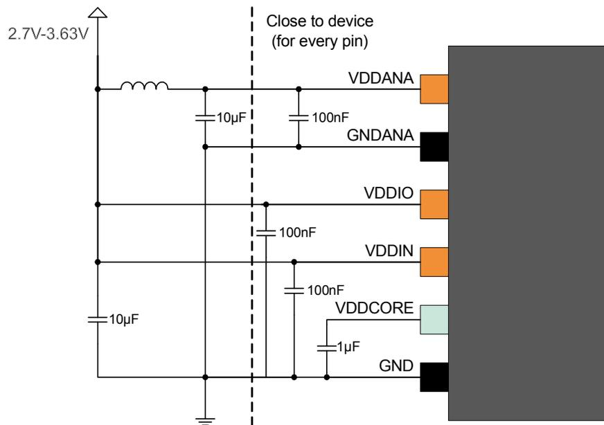
Table 41-1. Power Supply Connections,  $V_{\text{DDCORE}}$  From Internal Regulator
