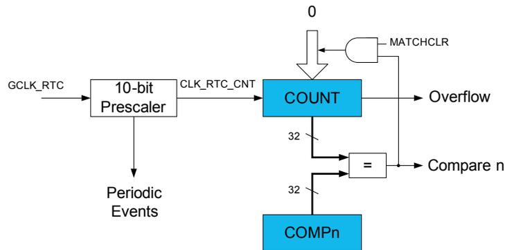
Figure 21-2. RTC Block Diagram (Mode 1 — 16-Bit Counter)
