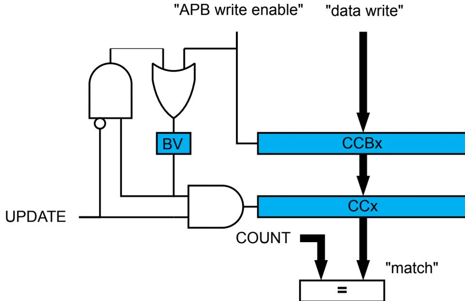
Both the registers (PATT/WAVE/PER/CCx) and corresponding buffer registers (PATTB/WAVEBV/PERB/CCBx) are available in the I/O register map, and the double buffering feature is not mandatory. The double buffering is disabled by writing a '1' to CTRLSET.LUPD.
