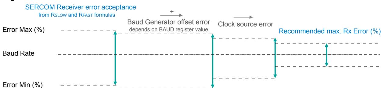
The recommendation values in the table above accommodate errors of the clock source and the baud generator. The following figure gives an example for a baud rate of 3Mbps:
