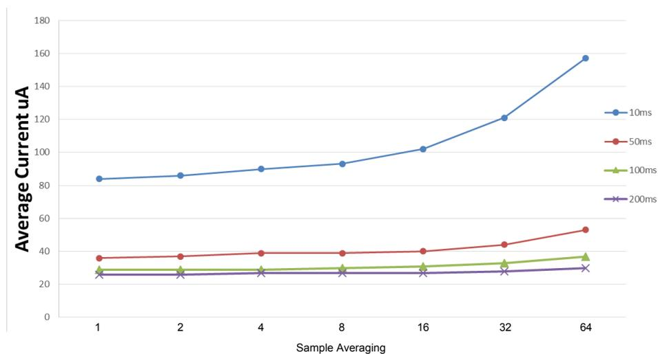
Figure 39-9. 10 Sensor / PTC\_GCLK = 4MHz / FREQ\_MODE\_NONE
