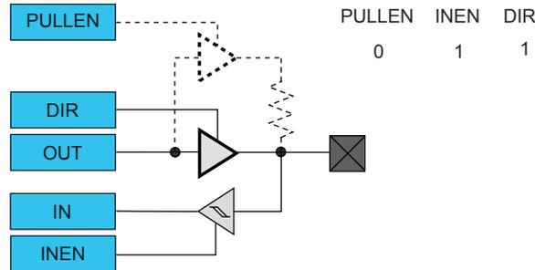
Figure 25-8. I/O Configuration - Output with Pull
