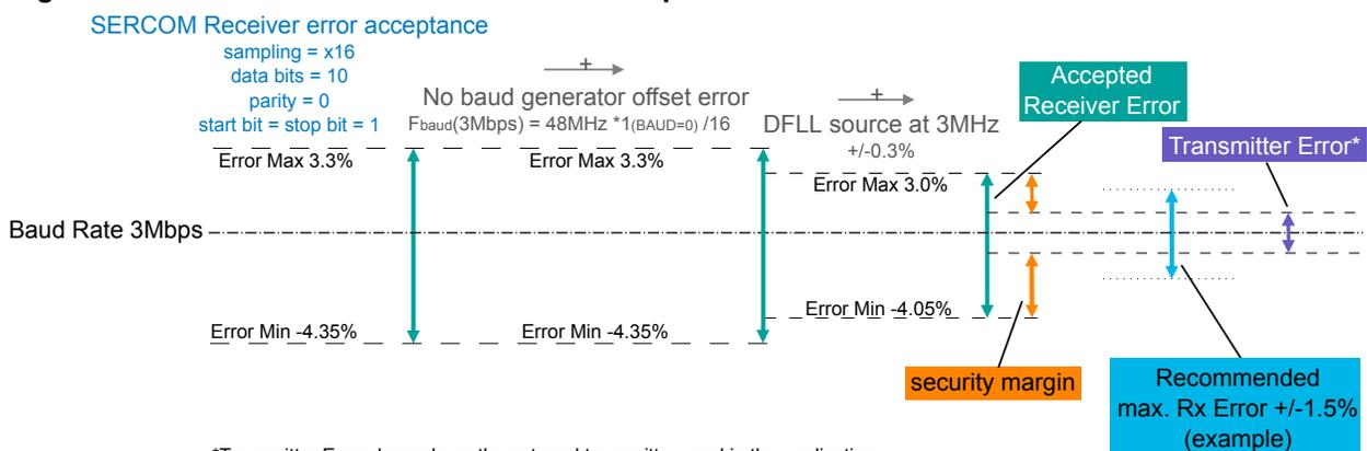
\*Transmitter Error depends on the external transmitter used in the application. It is advised that it is within the Recommended max. Rx Error (+/-1.5% in this example). Larger Transmitter Errors are acceptable but must lie within the Accepted Receiver Error.
