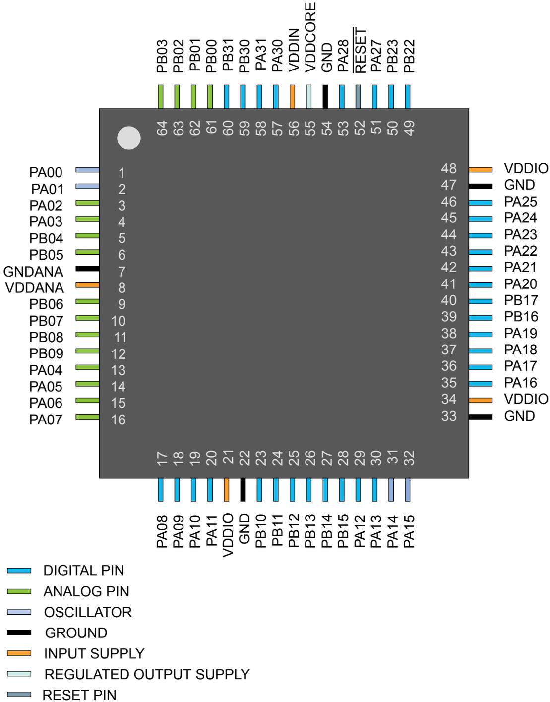
5.2 SAM DA1G - QFN48 / TQFP48
