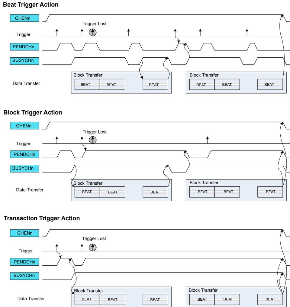
If the trigger source generates a transfer request for a channel during an ongoing transfer, the new transfer request will be kept pending ( $CHSTATUS.PEND=1$ ), and the new transfer can start after the ongoing one is done. Only one pending transfer can be kept per channel. If the trigger source generates more transfer requests while one is already pending, the additional ones will be lost. All channels pending status flags are also available in the Pending Channels register (PENDCH).
