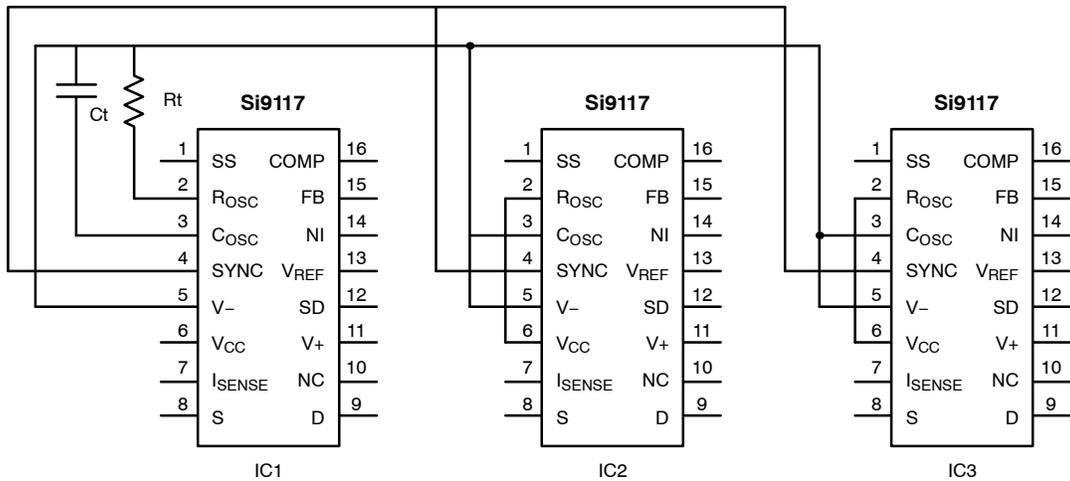
FIGURE 8. Oscillator Synchronization
