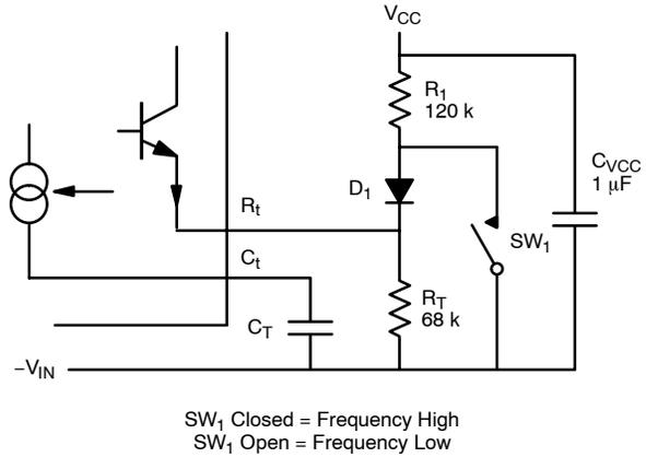
FIGURE 7. Frequency Shifting Using  $R_t$  Current Change
