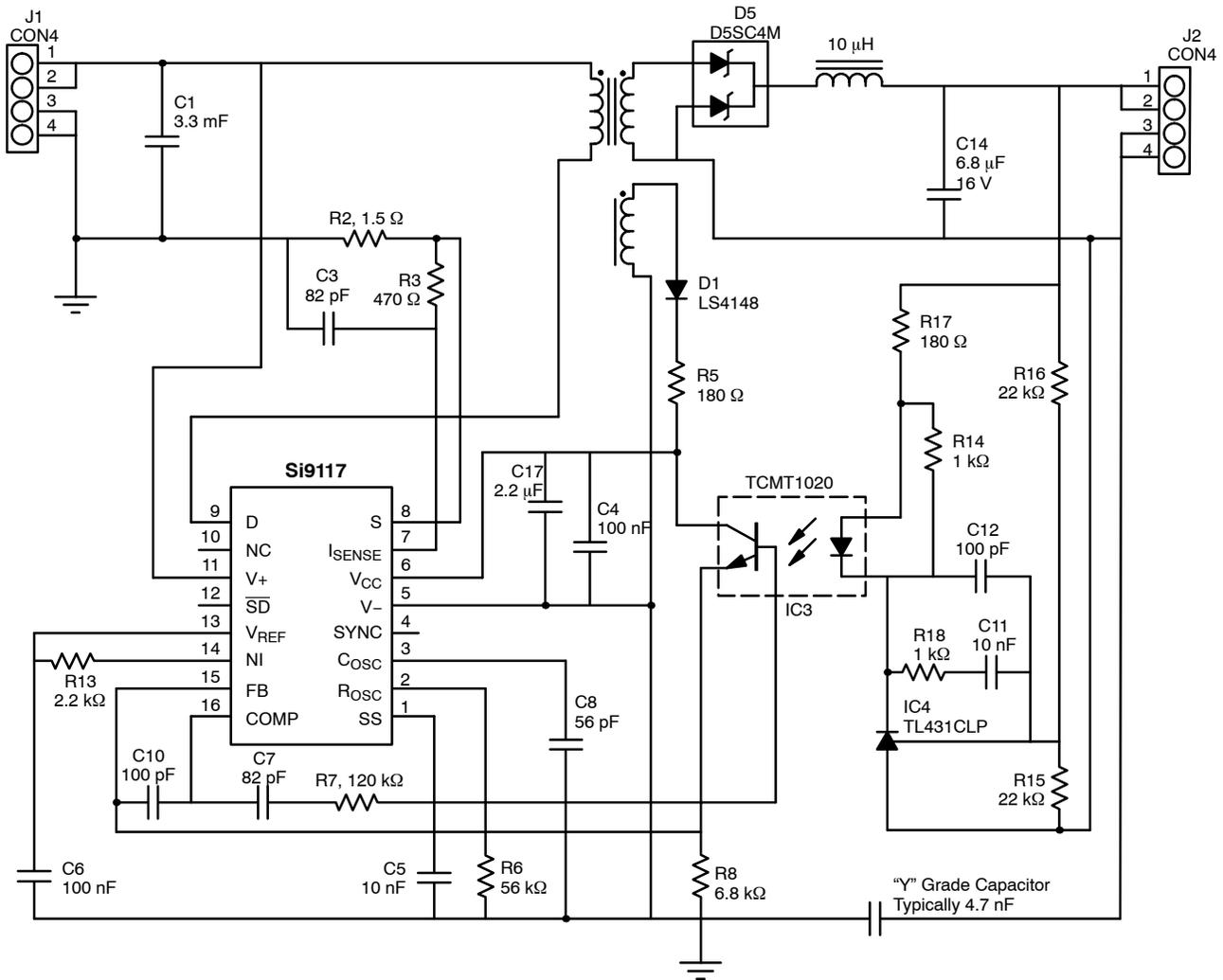
**FIGURE 15.** Complete Schematic Diagram
