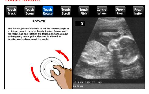
"Touch Rotate" is performed by rotating two touches about each other. It can be useful for rotating pictures, graphics or text on the screen.
