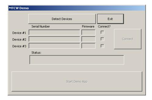
On the connect screen chose "Detect Devices" and a list of currently installed Grayhill Touch devices will appear. You'll likely have only one unit connected, and this device should appear under device #1. If it does not, check your USB cable and click "Detect Devices" once again.
