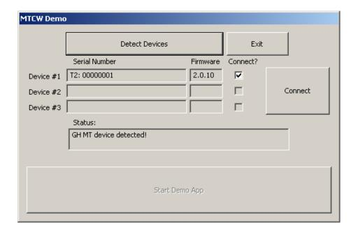
Next we'll need to connect to the device. After ensuring the "Connect?" checkbox next to the device that you wish to connect is checked, hit the "Connect" button. Notice the "Status:" changes to indicate that you are connected to the selected device.
